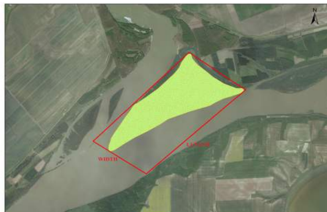
Figure 2. Example of fluvial islet in polygon format and the main parameters of them
